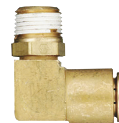
27205 Male Elbow Swivel 360° 3/8 Tube x 1/4 NPT
